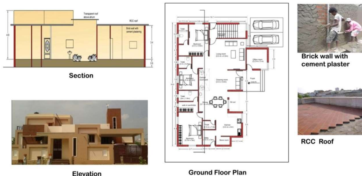
Figure 2: Conventional House with Reinforced Cement Concrete Roof / Brick wall with cement mortar
