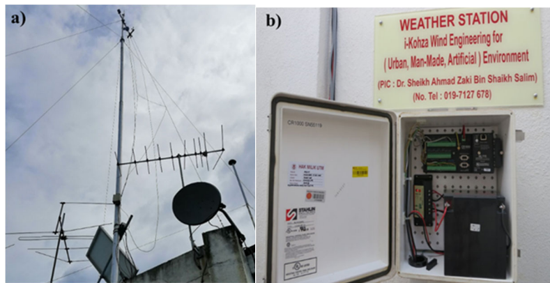
Figure 1. Weather station a) installed sensors and b) data logger at the rooftop of the MJIIT building.
