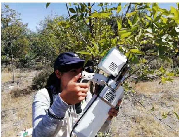
Figure 3: Measuring CO 2 assimilation using a Li-6800 portable photosynthesis equipment
