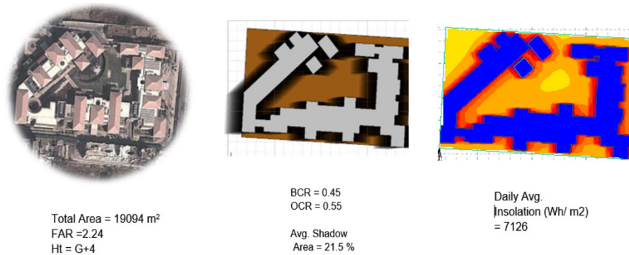
Figure7: Sample illustration of one location i) Existing satellite image and the spatial configuration ii) Shadow range on the hottest day of the year iii) Insolation graph
