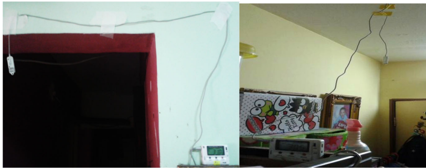
Figure 4. The installation of thermo recorder in each room.
